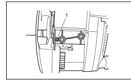
Adjusting the chain lubrication The engine must be switched off.
